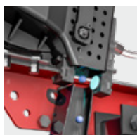
Light barrier for monitoring the planting process
